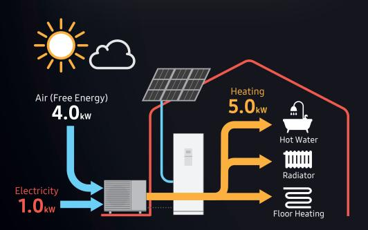
To generate 5.0kW of energy, it consumes only about 1kW of electricity and collects the rest from the air<sup>1</sup>.
