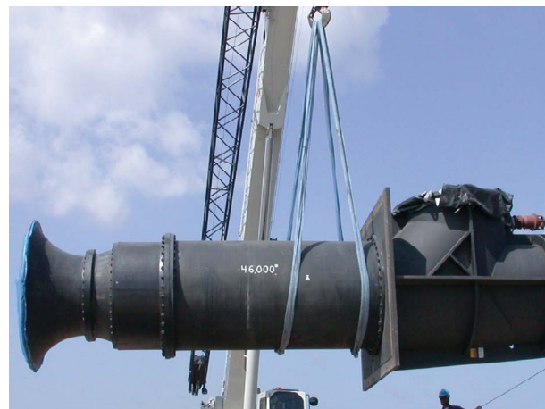
AC-series, Large vertical column pump
